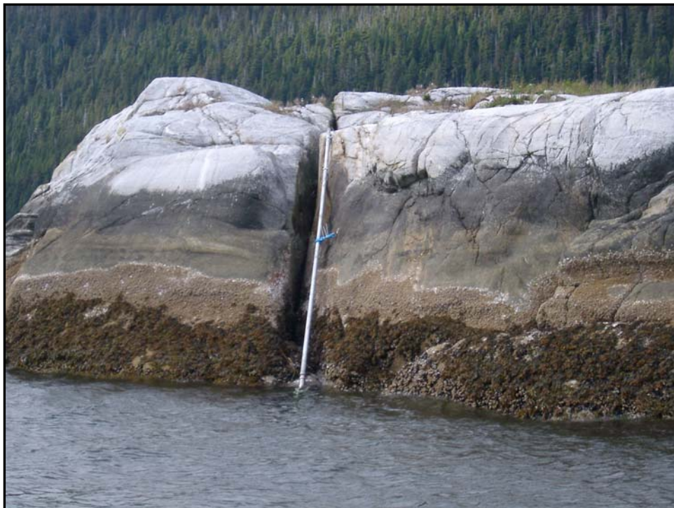
Photo 3: Emilia Rock Station Water Level Sensor
